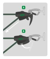
5. Pull excess line through tensioner [A] and close release handle [B].
