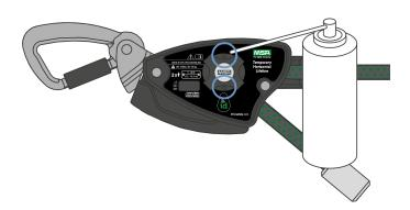
Moving parts of locking cam, carabiners and the tensioning handle may require periodic lubrication with low viscosity penetrating oil if movement is not smooth. Follow lubricant manufacturer's instruction. Do not over-lubricate. Wipe excess with a clean, dry cloth.
